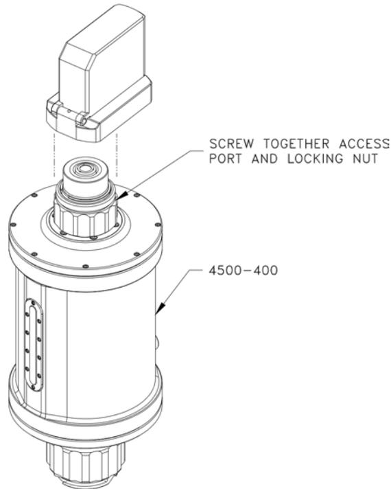
Figure 1-7. Attaching the wired access port to the VSM linear motor transport
