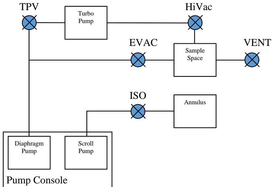
Figure C-2. Gas handling layout: MPMS 3 EverCool system
