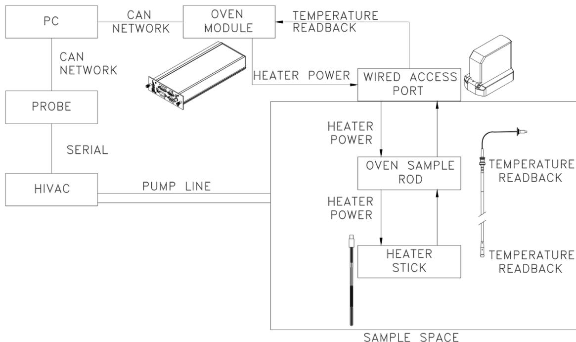
Figure 1-2. MPMS 3 Oven Option Block Diagram
