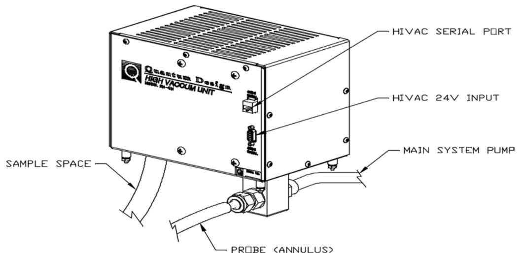
Figure 1-10. High Vacuum Unit (Model EM-QM)
