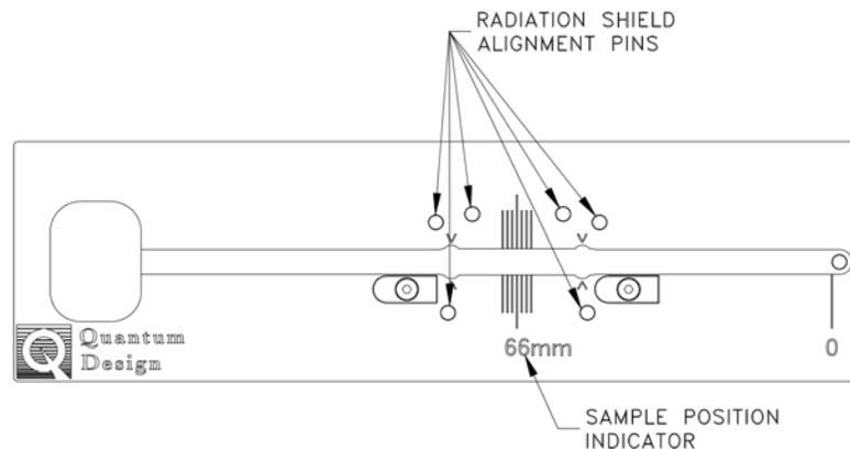
Figure 1-12. MPMS 3 Oven sample mounting platform
