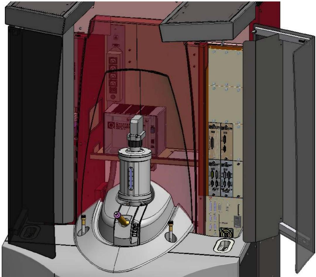
Figure 1-1. MPMS 3 VSM system installed with MPMS 3 Oven Option
