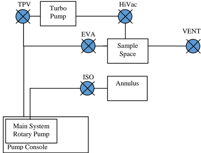
Figure C-1. Gas handling layout: Standard MPMS 3 system
