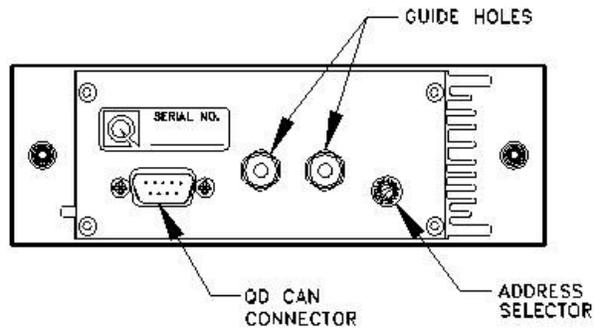
Figure 1-9. Back Panel of the Model CM-C VSM Oven module
