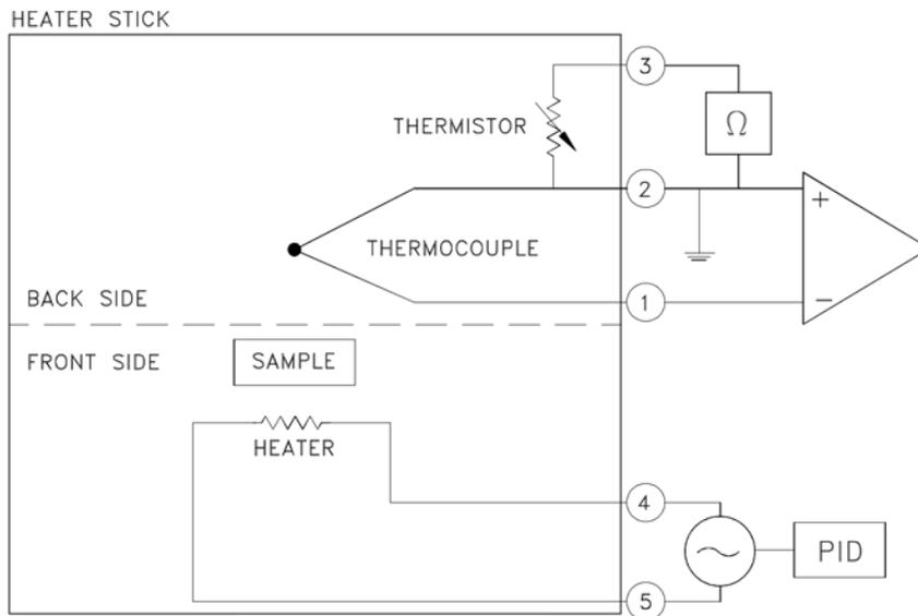
Figure 1-3. Control circuit for the Oven heater stick
