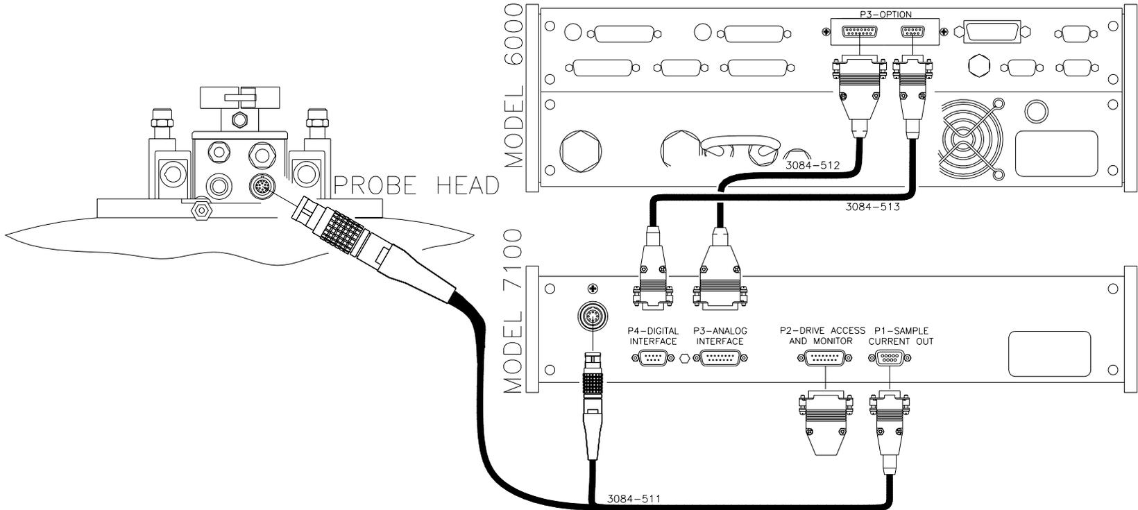
See connection diagrams for cabling with rotator and He3
