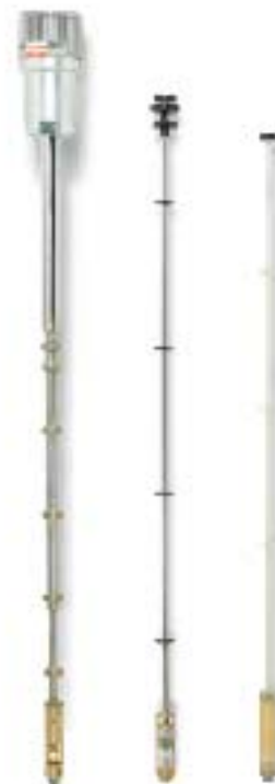
Different PPMS application inserts. From left to right: Helium-3, Horizontal Rotator, and ACMS.
