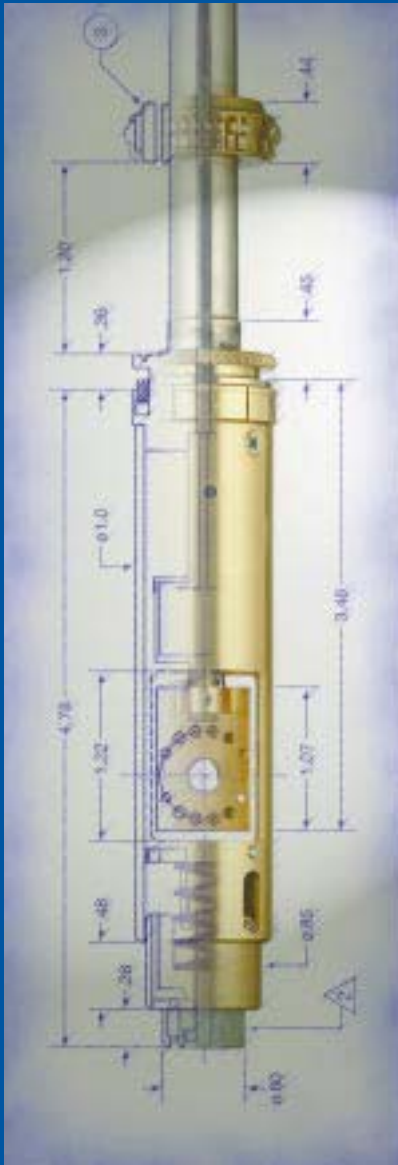
A new concept in refrigeration design, this self-contained 3 He Refrigerator lowers the minimum sample temperature to < 0.4 K.
