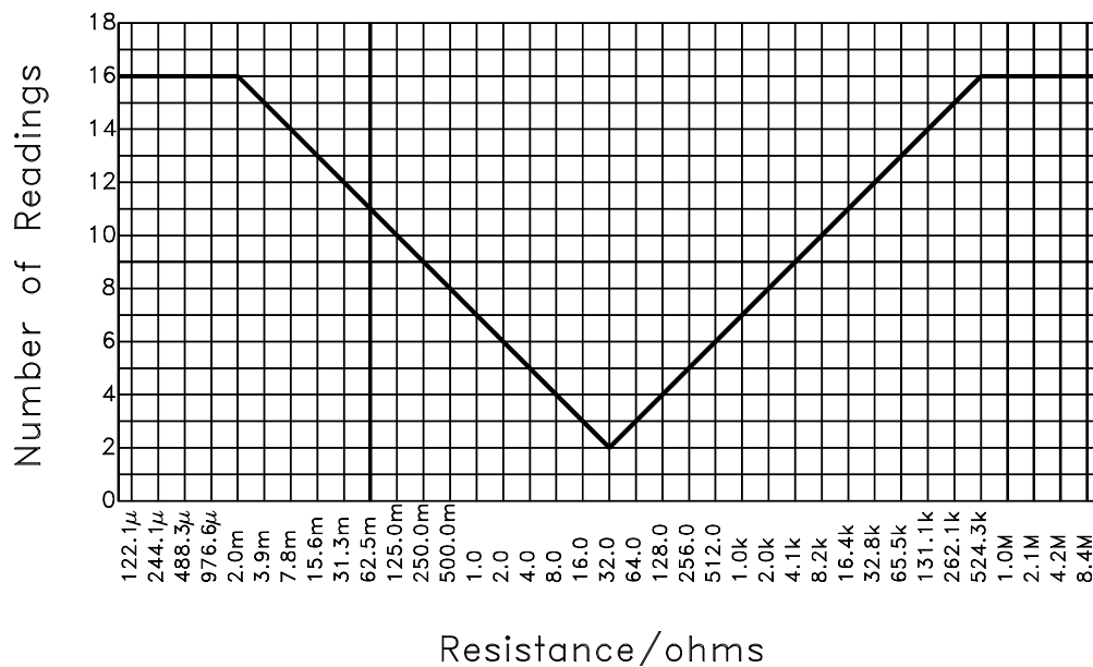
Figure 2-2. The number of measurements averaged in high-resolution mode varies from 2 to 16 and depends on how far from the base value of 32.767 \Omega the resistance lies. Non-integers on the y-axis are rounded down in this graph.
