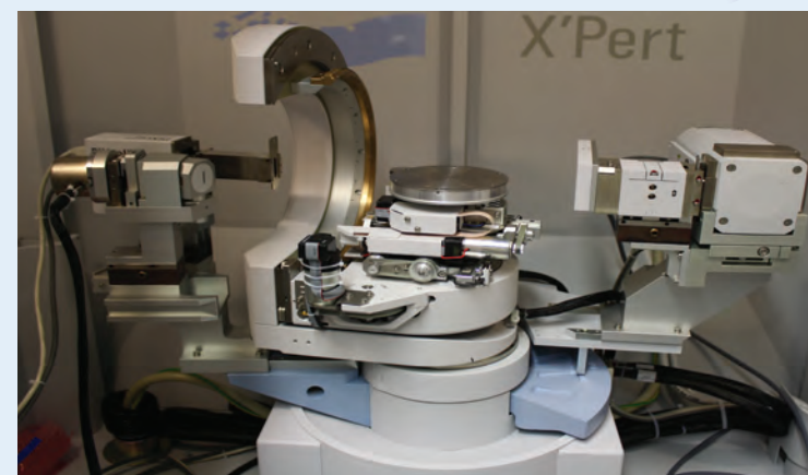
The X-Ray and TEMPO Facilities provide diffraction tools for characterizing the structural properties of a wide range of materials.
