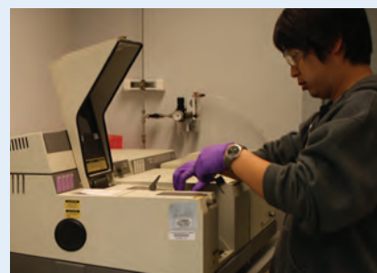
The FTIR/Raman Spectrometer probes chemical bonds and structure in molecular materials.
