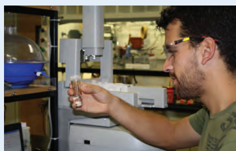
Microwave reactors in the Polymer Facility create controlled conditions for monomer synthesis and polymerizations.
