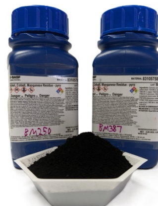
‘Black mass’ is the complex mix of compounds resulting from the pyrolysis of LIBs.
