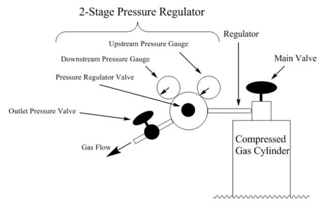
Clockwise Turning = Shutting Off/Reducing Gas Flow
