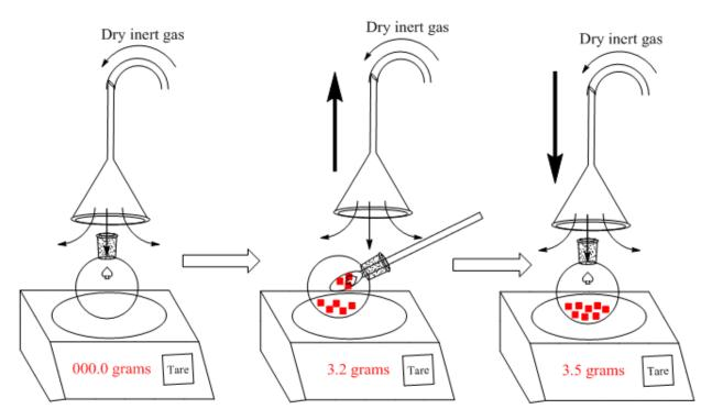
The inverted funnel technique can also be used for manipulating air/water reactive materials in odd-shaped and/or irregular pieces of equipment (e.g., pressure tubes, Büchner funnels, beakers, reaction kettles).
