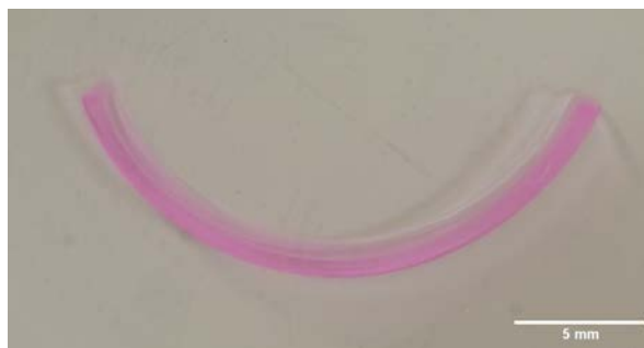
Polyacrylamide hydrogel synthesized against heterogeneous substrates demonstrates curvature after swelling in water (unpublished data).
