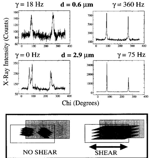
Fig. 6. X-ray diffractograms of 8CB confined between soft surfaces at different gaps and shear rates. These one-dimensional scans were derived from 2D images. (Top) The gap is  $6000\ \text{\AA}$  for shear rates of 18 and 360 Hz. (Middle) The gap is  $2.9\ \mu\text{m}$  with shear rates of 0 and 75 Hz. In both cases, it can be seen that shear aligns the smectic domains significantly. (Bottom) Schematic of the domain orientation occurring as a function of shear.
