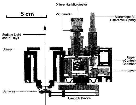
Fig. 3. Schematic of the X-Ray Surface Forces Apparatus without the lower sealed chamber. The two micrometers used for varying the gap can be seen at the top of the device, while the piezoelectric bimorph shearing device is on the bottom. Figure adapted from Ref. [24].
