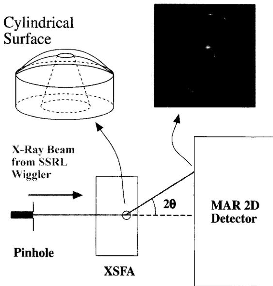
Fig. 5. Schematic of the XSFA experimental setup. X-rays from Stanford Synchrotron Radiation Laboratory wiggler beamline 6-2 impinge on a  $125\ \mu\text{m}$  pinhole to produce a high resolution setup. The X-rays then scatter off the sample confined between cylindrical surfaces into an MAR two-dimensional image plate detector to yield a diffraction pattern showing the sample alignment.
