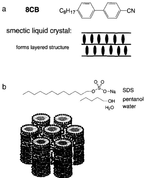
Fig. 1. The two systems studied in this work are the smectic liquid crystals 8CB (4-cyano-4'-octylbiphenyl) which forms a layered smectic phase at room temperature, and a lyotropic liquid crystalline mixture of sodium dodecyl sulfate (SDS), water and pentanol which forms an hexagonal phase at room temperature.
