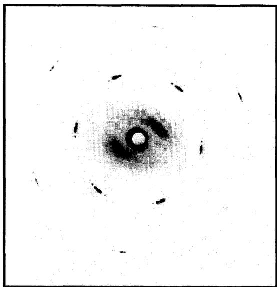
Fig. 7. Two-dimensional X-ray diffractogram of the SDS lyotropic liquid crystal sample illustrating the beautiful six-fold hexagonal symmetry. The shadow near the beam stop comes from the scattering of the mylar mirrors used for optical access to the sample.
