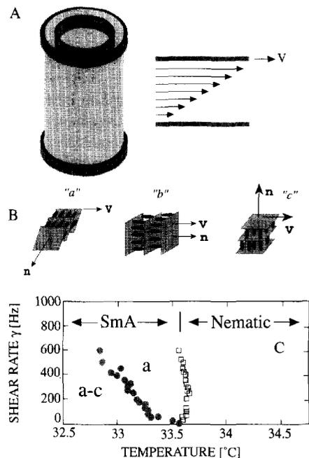
Fig. 2. Bulk shear flow experiments conducted in an X-Ray couette shear cell shown in (A) with a velocity profile between the two cylinders as shown. The three orthogonal orientations of a layered system between two sliding surfaces are shown in (B). (C): shear rate-temperature phase diagram of 8CB under flow showing the absence of the  $b$  orientation [19].
