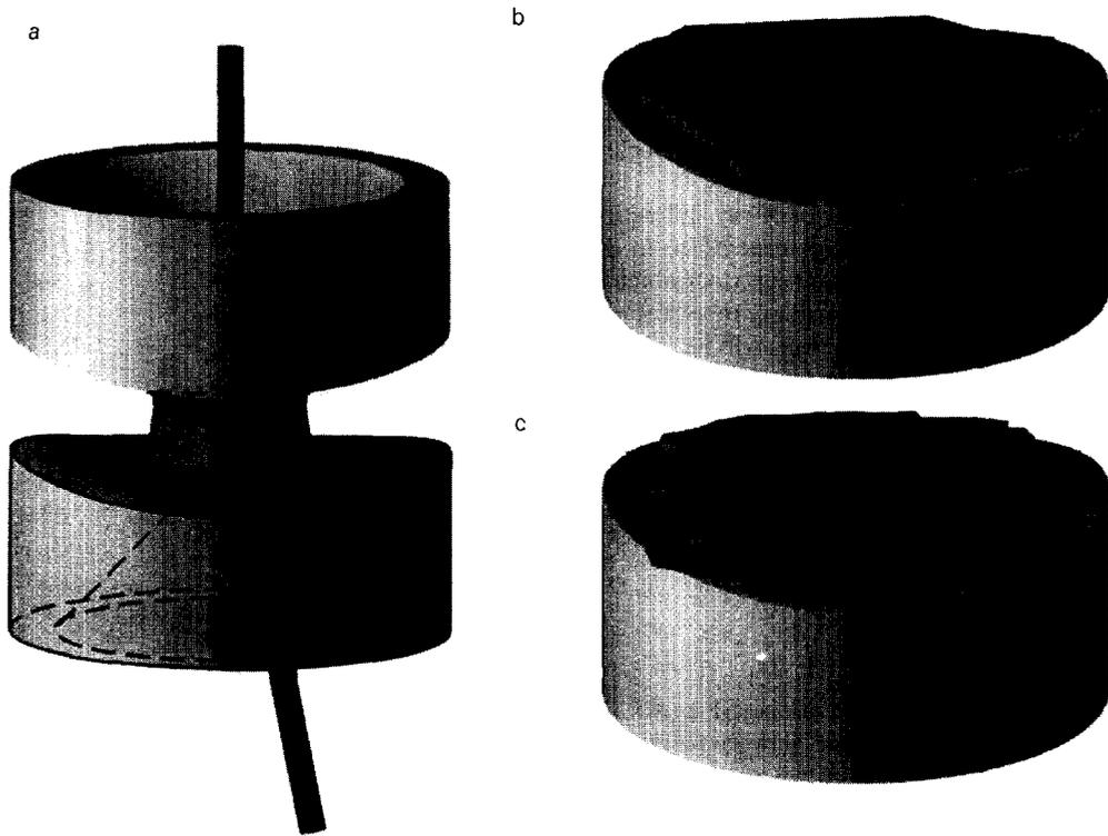
Fig. 4. (a) Surface geometry in an XSFA experiment showing the X-rays scattered by a sample confined between two cylindrical surfaces (disk mounts). (b) "Soft surfaces" consisting of a thin mica sheet ( $\sim 3\text{--}5\ \mu\text{m}$  thick) glued to the disk surface only around the central hole. (c) "Hard surfaces" are constructed by first gluing a thin sheet of quartz glass over the hole, followed by the mica sheet.
