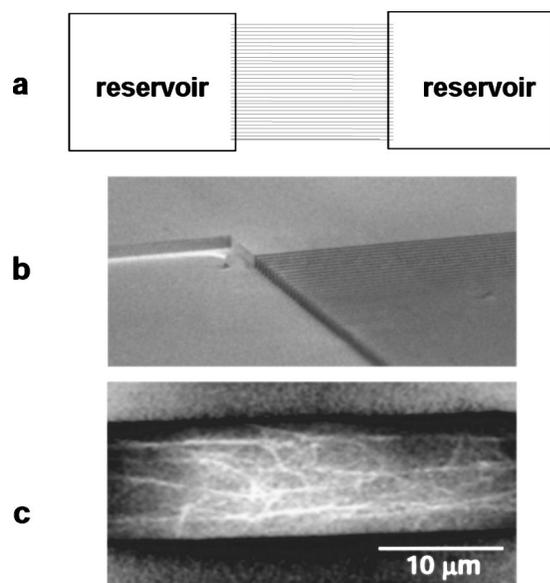
FIG. 2. (a) Schematic layout of the microchannel device. (b) SEM image of a section of the device; (c) fluorescence micrograph of 0.1 mg/ml actin bundled with 0.1 mg/ml  $\alpha$ -actinin inside a single 10- $\mu\text{m}$ -wide  $\times$  10- $\mu\text{m}$ -deep-channel. The bundles are predominantly aligned parallel to the channel.
